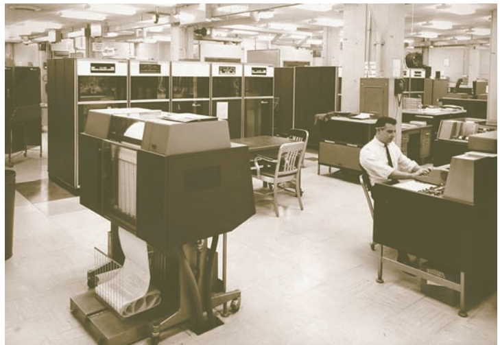
Figure 2. NSA in the 1960s relied on the IBM 7030 Stretch connected to the one-of-a-kind HARVEST unit, which was operational in 1962 (shown here in 1968). 33
