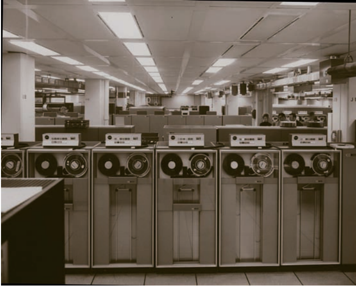
Figure 1. National Security Agency's Univac 494 and the time-sharing RYE computing system. 33 A color version dated 1972 appears online in an article by James Bamford. 34
